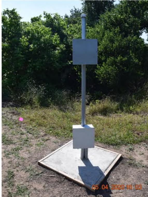
The installed telemetry system. The upper box contains the telemetry unit and the lower box houses excess lengths of installed system cables.
