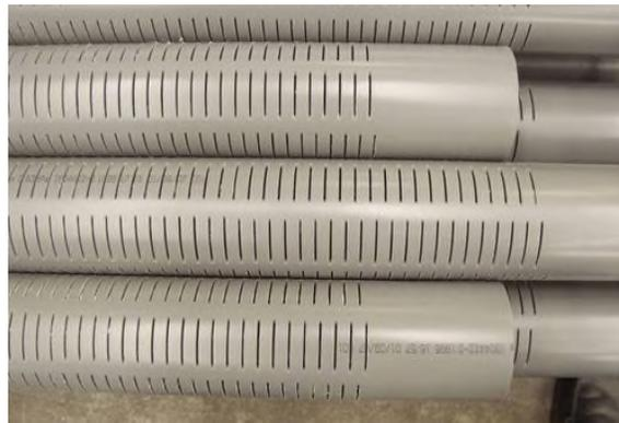
The monitor wells were constructed using 2-inch PVC slotted pipe (shown in the lower picture) within the alluvial aquifer and solid 2-inch PVC pipe from the aquifer to the about 2 feet above ground level at each well location. The above-ground portion of the PVC pipe was protected with a 4-inch square lockable steel enclosure.
