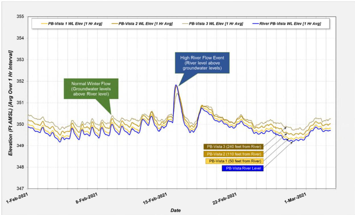
Figure 14. Water Level Elevation Response Delay
