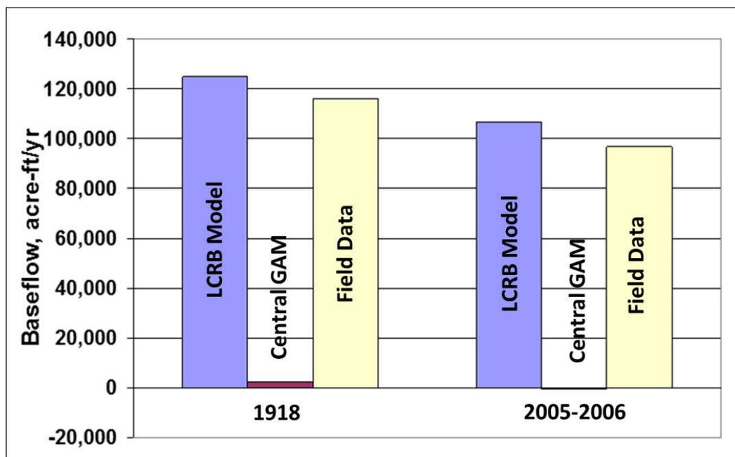
**Figure 4.** Comparison of measured baseflow along the Colorado River (Field Data) with simulated baseflow values from the LCRB groundwater model and from the Central Gulf Coast Groundwater Availability Model (data from Young et al. 2009; LCRB = Lower Colorado River Basin, GAM = groundwater availability model). The Field Data includes gain-loss studies performed with river gage data reported by Slade (2002) and Saunders (2006).
