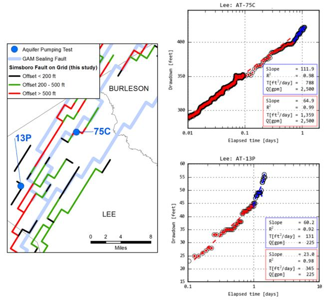
Figure 3.1.4.1d. Location of aquifer pumping tests near faults in Lee County that produced a CJSLcalculated late-time transmissivity value less than the early-time transmissivity value, which provides a line of evidence that faults could be affecting groundwater flow. For aquifer tests AT-75C and AT-13P, the values for the late-to early-time transmissivity ratio are 0.58 and 0.38, respectively.
