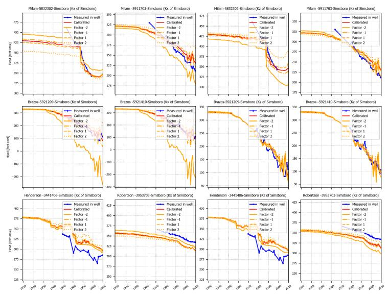
Figure 6.2.2x. Hydrographs showing sensitivity of heads (in feet above mean sea level) to changes in the horizontal and vertical hydraulic conductivity of the Simsboro Formation for select wells completed in the Simsboro Formation.
