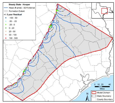
Figure 5.3.400. Contours in feet (ft) above mean sea level (amsl) developed from simulated hydraulic heads for steady-state conditions in the Hooper Formation with residuals posted.
