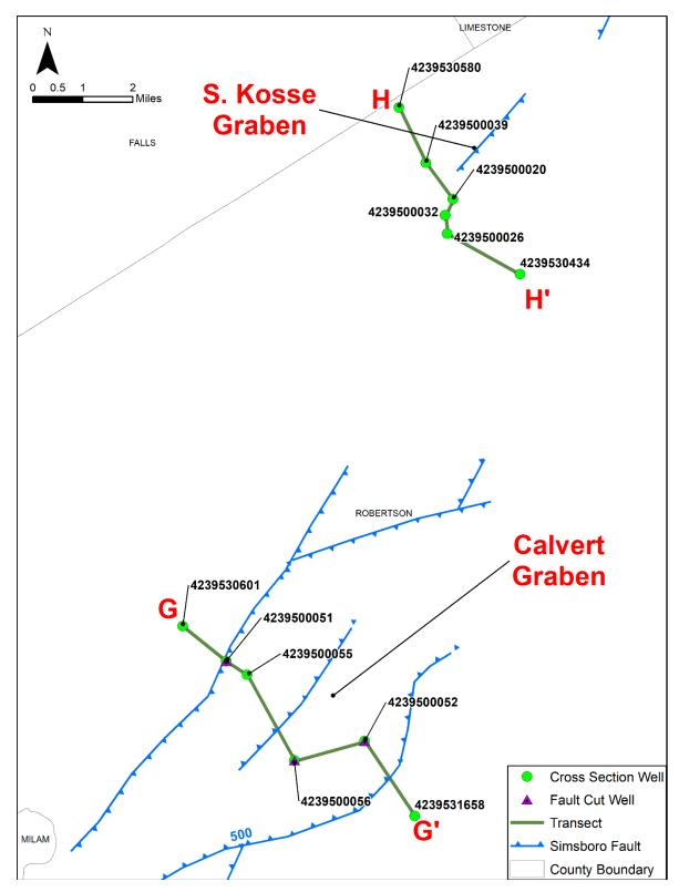
Figure 3.1.2.4a. Simsboro Formation faults and estimated fault offset (in feet) in the South (S.) Kosse and Calvert Grabens in Robertson County. Fault arrows point to the down-thrown side of the fault. The wells are labeled with their American Petroleum Institute number.
