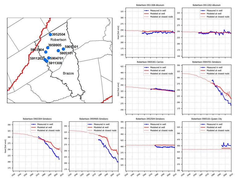
Figure 5.3.6c. Hydrographs showing simulated and measured hydraulic heads (in feet above mean sea level) in the Brazos Valley Groundwater Conservation District at eight wells with state well numbers 5911308, 5911202, 05905301, 05904701, 05903304, 03959905, 03952504, 03952504, 03952504, 05905101.
