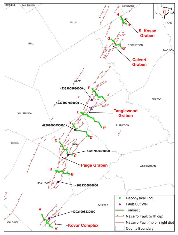
Figure 3.1.2g. Plan view map of the Milano Fault Zone showing the five named major areas of faulting, locations of cross-sections that transect the fault zone, and locations of fault cut wells shown in Figure 3.1.2d.
