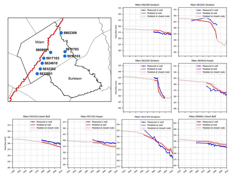
Figure 5.3.6a. Hydrographs showing simulated and measured hydraulic heads (in feet above mean sea level) in the Post Oak Savannah Groundwater Conservation District at eight wells with state well numbers 5902309, 5832501, 5832302, 5824610, 5911703, 5917103, 5911402, and 5909901.
