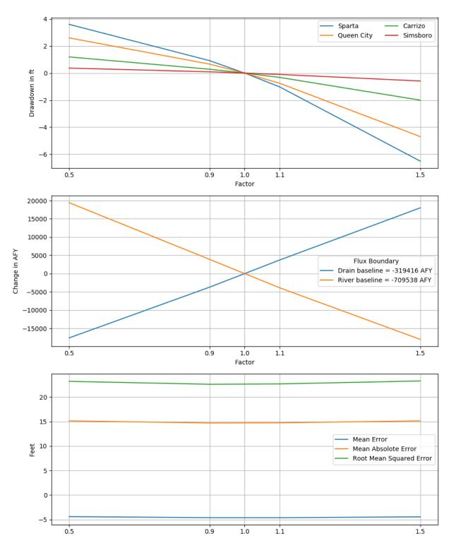
Figure 6.2.2a. Sensitivities of 2010 drawdown in hydrogeologic units (top), hydraulic boundary fluxes (center), and calibration statistics (bottom) to the horizontal hydraulic conductivity of the Sparta Aquifer for the transient model.
