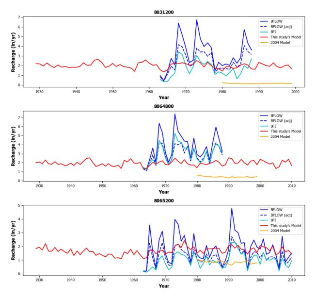
Figure 5.4.2aComparison of recharge rates (in inches per year) calculated from base flow for river<br/>gages 8031200, 8064800, and 8065200 based on the Baseflow Program analysis and<br/>adjusted Baseflow Program values, the Base Flow Index Program analysis, and calculated<br/>from this study's model and the 2004 groundwater availability model by Kelley and others<br/>(2004). The model values equal the model calculated discharge to rivers/streams.
