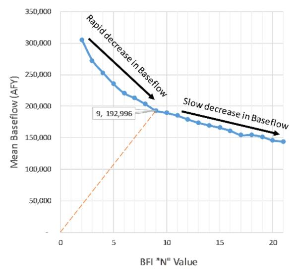
Figure 3.3.2.1b. Mean base flow from the Base Flow Index Program (BFI) analysis for river gage 08041500 for different values of the *N* parameter, which shows that the greatest change in slope occurs for an *N* value of 9.
