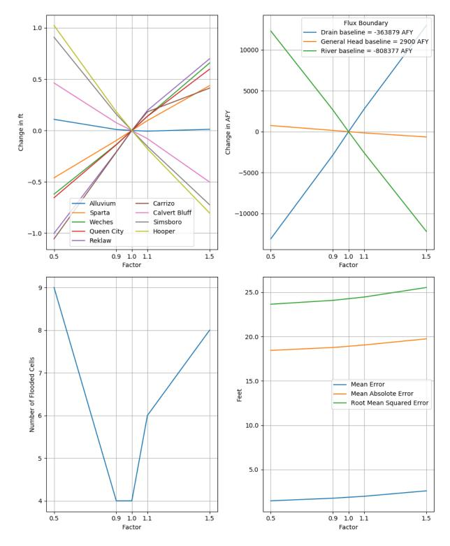
Figure 6.2.1k.Sensitivity of averaged hydraulic head in hydrogeologic units (top left), hydraulic<br/>boundary fluxes (top right), additional flooded grid cells (bottom left), and calibration<br/>statistics (bottom right) to the horizontal hydraulic conductivity of the Carrizo Aquifer for<br/>the steady-state model.
