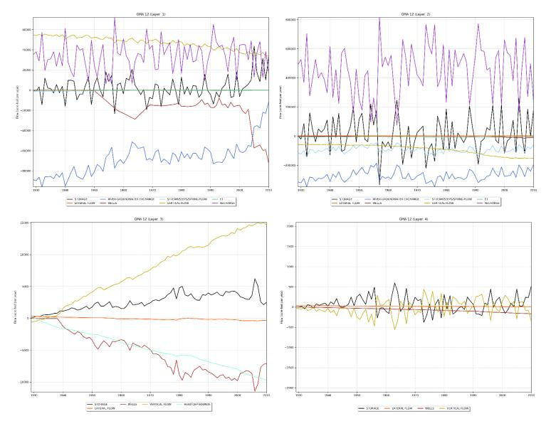
Figure 5.5.2d. Transient water budget for Groundwater Management Area 12 for model layers 1, 2, 3, and 4.
