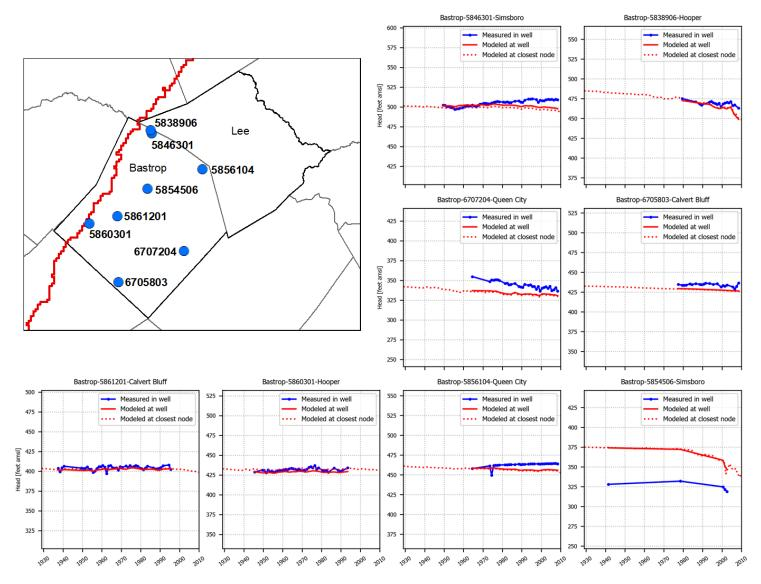
Figure 5.3.6f. Hydrographs showing simulated and measured hydraulic heads (in feet above mean sea level) in the Lost Pines Groundwater Conservation District at eight wells with state well numbers 5846301, 5838906, 6707204, 6705803, 5861201, 5860301, 5856104, and 5854506.
