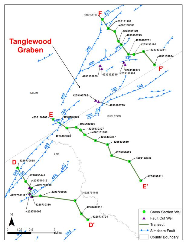
Figure 3.1.2.3a. Simsboro Formation faults and estimated fault offset (in feet) in the Tanglewood Graben in Lee, Milam and Burleson counties. Fault arrows point to the down-thrown side of the fault. The wells are labeled with their American Petroleum Institute number.
