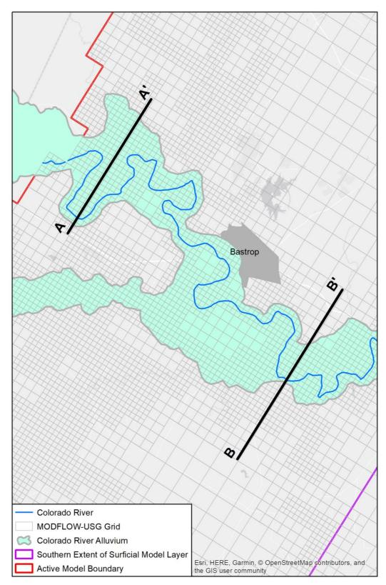
Figure 3.4.1a. Areal extent of the Colorado River alluvium mapped onto the numerical grid for the updated groundwater availability model for the central portion of the Carrizo-Wilcox, Queen City, and Sparta aquifers.
