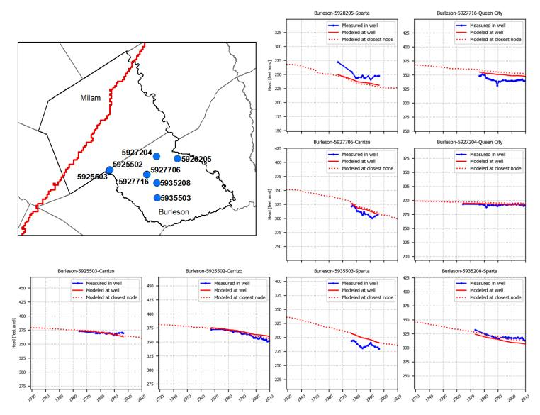
Figure 5.3.6b. Hydrographs showing simulated and measured hydraulic heads (in feet above mean sea level) in the Post Oak Savannah Groundwater Conservation District at eight wells with state well numbers 5928205, 5927716, 5927706, 5927204, 5925503, 5925502, 5935503, 5935208.
