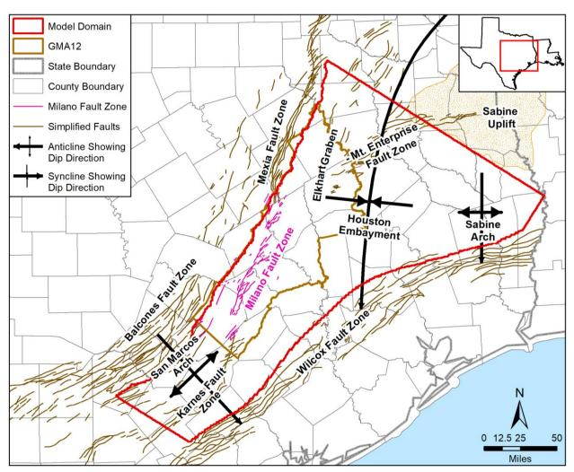
Figure 2.4a.Map of major faults and structural features in the vicinity of the model area. Wilcox and<br/>Balcones Fault Zones modified from Ewing and others (1990), Milano Fault Zone<br/>developed by this study; and structural axes modified from Guevara and Garcia (1972),<br/>Galloway (1982), and Galloway and others (2000).
