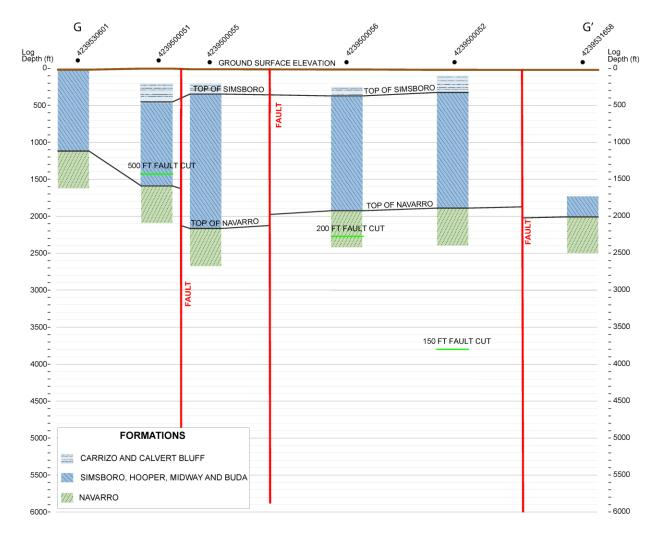
Figure 3.1.2.4b. Cross-section G-G' through the Calvert Graben showing the top surface of selected formations and mapped fault locations based on interpretation of geophysical logs in and near cross-section G-G'.
