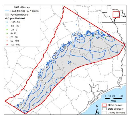
Figure 5.3.40. Contours in feet (ft) above mean sea level (amsl) developed from simulated hydraulic heads for 2010 in the Weches Formation with residuals posted.
