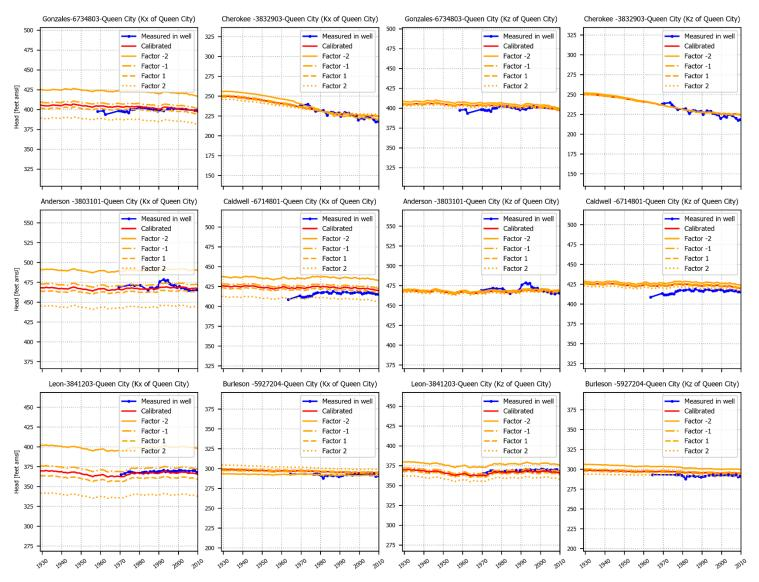
Figure 6.2.2v. Hydrographs showing sensitivity of heads (in feet above mean sea level) to changes in the horizontal and vertical hydraulic conductivity of the Queen City Aquifer for select wells completed in the Queen City Aquifer.
