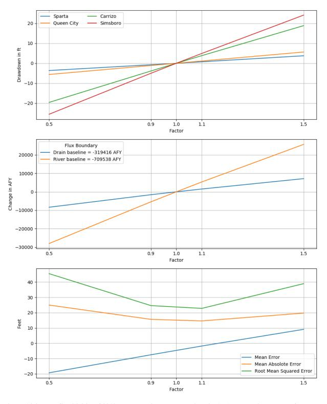
Figure 6.2.2t.Sensitivities of 2010 drawdown in hydrogeologic units (top), hydraulic boundary fluxes<br/>(center), and calibration statistics (bottom) to the pumping rate for the transient model.
