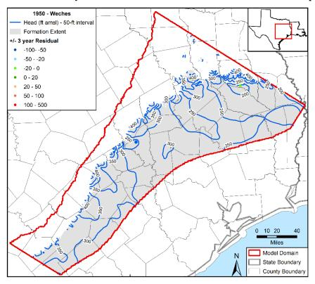
Figure 5.3.41. Contours in feet (ft) above mean sea level (amsl) developed from simulated hydraulic heads for 1950 in the Weches Formation with residuals posted.
