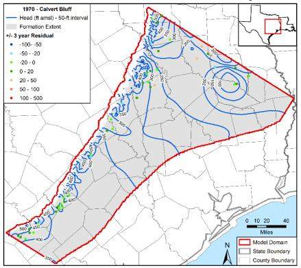
Figure 5.3.4gg. Contours in feet (ft) above mean sea level (amsl) developed from simulated hydraulic heads for 1970 in the Calvert Bluff Formation with residuals posted.
