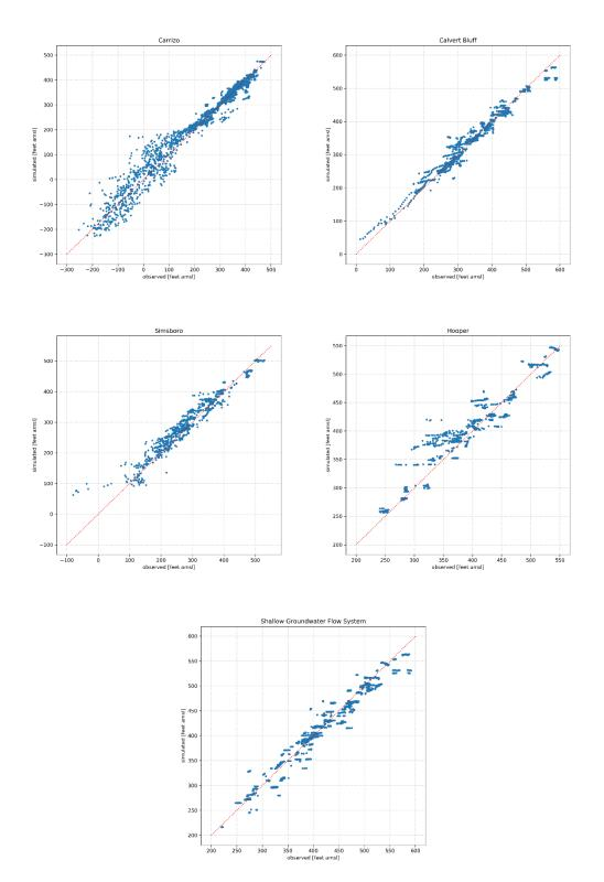
Figure 5.3.3j. Scatter plots of simulated versus observed hydraulic heads for all calibration targets in all wells in the Carrizo Aquifer, the Calvert Bluff Formation, the Simsboro Formation, the Hooper Formation and the shallow groundwater flow system for the transient period 1930 to 2010.
