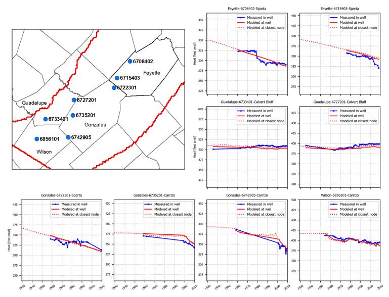
Figure 5.3.6i. Hydrographs showing simulated and measured hydraulic heads (in feet above mean sea level) in the Fayette County Groundwater Conservation District and Groundwater Management Area 13 at eight wells with state well numbers 6708402, 6715403, 6733401, 6727201, 6722301, 6735201, 6742905, and 6856101.
