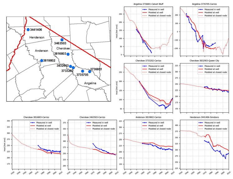
Figure 5.3.6j. Hydrographs showing simulated and measured hydraulic heads (in feet above mean sea level) in Groundwater Management Area 11 at eight wells with state well numbers 3736801, 3935705, 3733202, 3832903, 3816803, 3463503, 3819802, and 3441406.
