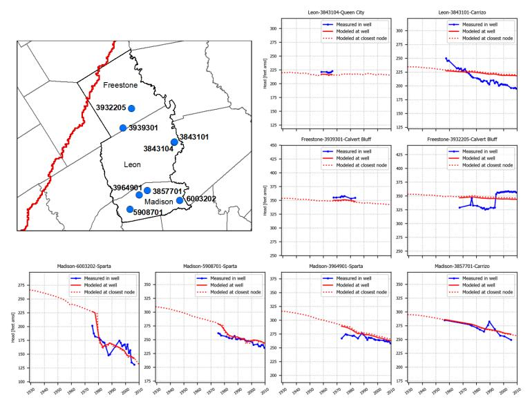
Figure 5.3.6g. Hydrographs showing simulated and measured hydraulic heads (in feet above mean sea level) in the Mid-East Texas Groundwater Conservation District at eight wells with state well numbers 3843104, 3843101, 3939301, 3932205, 6003202, 5908701, 3964901, and 3857701.
