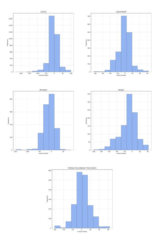
Figure 5.3.31. Histograms of the hydraulic head residuals for all calibration targets in all wells in the Carrizo Aquifer, the Calvert Bluff Formation, the Simsboro Aquifer, the Hooper Aquifer, and the shallow groundwater flow system for the transient period 1930 to 2010.
