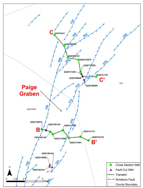
Figure 3.1.2.2a. Simsboro Formation faults and estimated fault offset (in feet) in the Paige Graben in Bastrop and Lee counties. Fault arrows point to the down-thrown side of the fault. The wells are labeled with their American Petroleum Institute number.
