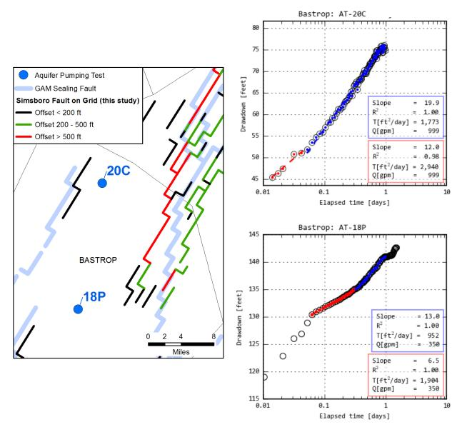
Figure 3.1.4.1e. Location of aquifer pumping tests near faults in Bastrop County that produced a CJSLcalculated late-time transmissivity value less than the early-time transmissivity value, which provides a line of evidence that faults could be affecting groundwater flow. For aquifer tests AT-20C and AT-18P, the values for the late-to early-time transmissivity ratio are 0.60 and 0.50, respectively.
