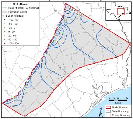
Figure 5.3.4ss. Contours in feet (ft) above mean sea level (amsl) developed from simulated hydraulic heads for 2010 in the Hooper Formation with residuals posted.
