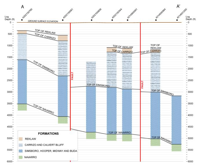
Figure 3.1.2.1b. Cross-section A-A' through the Kovar Complex showing the top surface of selected formations and mapped fault locations based on interpretation of geophysical logs in and near cross-section A-A'.
