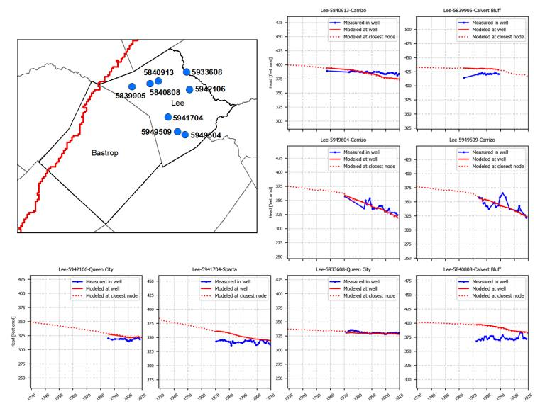
Figure 5.3.6e. Hydrographs showing simulated and measured hydraulic heads (in feet above mean sea level) in the Lost Pines Groundwater Conservation District at eight wells with state well numbers 5840913, 5839905, 5949604, 5949509, 5942106, 5941704, 5933608, and 5840808.
