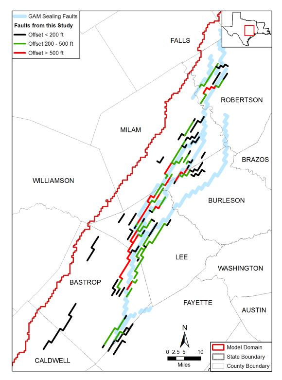
Figure 3.1.3a. Sealing faults in the groundwater availability model (GAM) for the central portion of the Carrizo-Wilcox, Queen City, and Sparta aquifers and the Simsboro Formation faults from this study sampled onto the groundwater availability model grid and color-coded based on the amount of offset between the Simsboro Formation updip and downdip of the fault.
