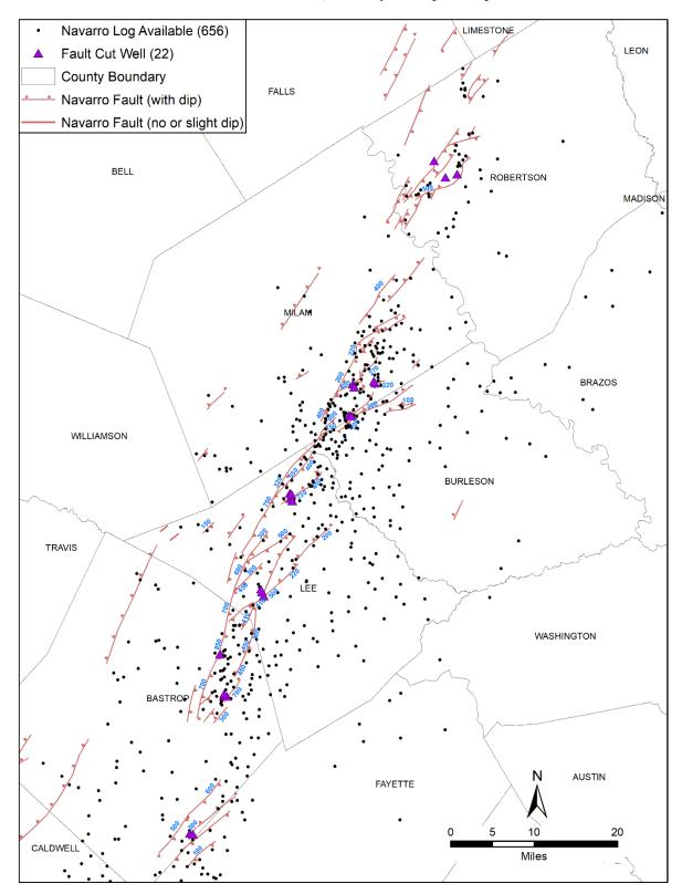
Figure 3.1.2b. Faults mapped onto the top of the Navarro Group determined primarily from the top of the Navarro Group picks from 656 geophysical logs with fault traces mapped on Geologic Atlas of Texas sheets (Barnes, 1970, 1979, 1981). Fault arrows point to the down-thrown side of the fault. Numerical values indicate fault offset in feet.
