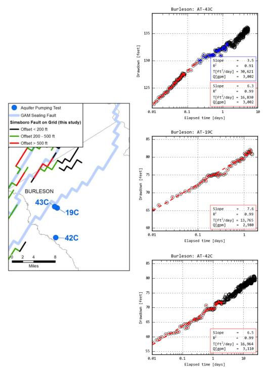
Figure 3.1.4.1f. Location of aquifer pumping tests near faults in Burleson County that produced a CJSLcalculated late-time transmissivity value equal to or greater than the early-time transmissivity value, which provides little evidence that faults could be affecting groundwater flow. For aquifer tests AT-43C, AT-19C, and AT-42C, the values for the lateto early-time transmissivity ratio are 1.82, 1.0, and 1.0, respectively.
