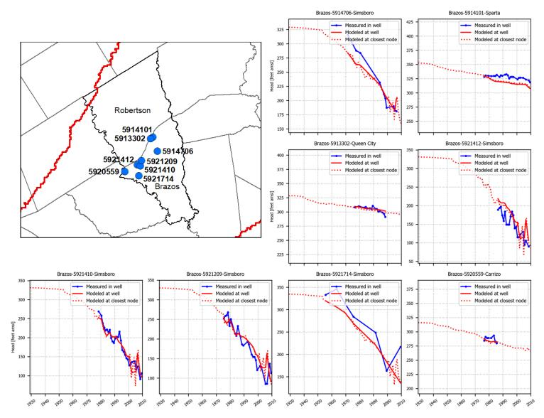
Figure 5.3.6d. Hydrographs showing simulated and measured hydraulic heads (in feet above mean sea level) in the Brazos Valley Groundwater Conservation District at eight wells with state well numbers 5914706, 5914101, 5913302, 5921412, 5921410, 5921209, 5921714, and 5920559.
