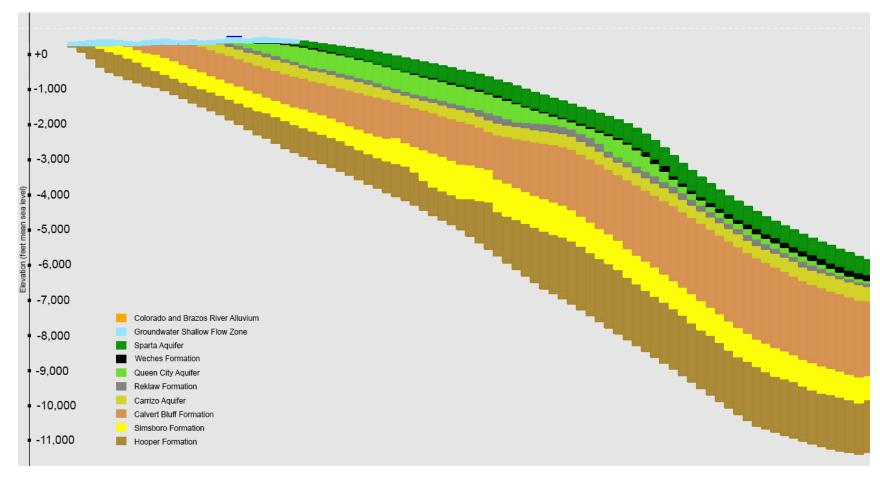
Figure 4.2.1n. Vertical cross-section showing the model layers along dip cross-section B-B'.
