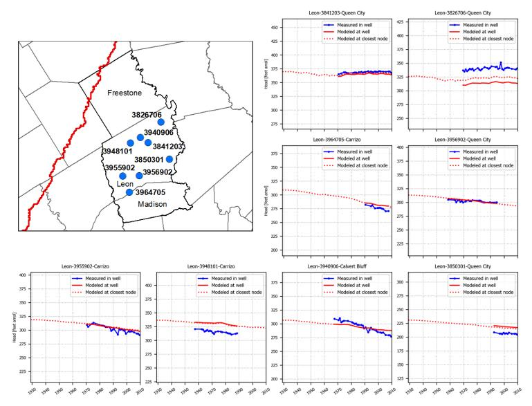
Figure 5.3.6h. Hydrographs showing simulated and measured hydraulic heads (in feet above mean sea level) in the Mid-East Texas Groundwater Conservation District at eight wells with state well numbers 3841203, 3826706, 3964705, 3956902, 3955902, 3948101, 3940906, and 3850301.
