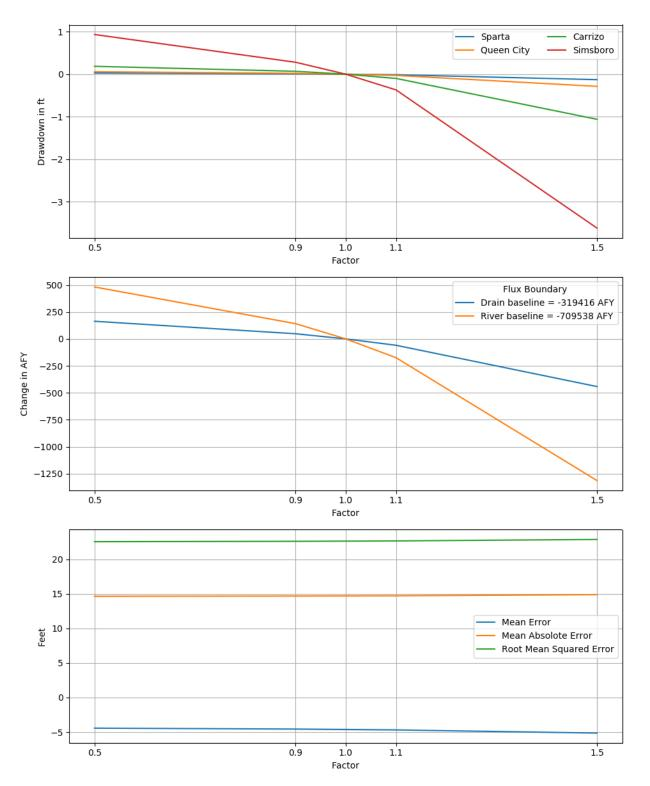
Figure 6.2.20. Sensitivities of 2010 drawdown in hydrogeologic units (top), hydraulic boundary fluxes (center), and calibration statistics (bottom) to the specific storage of the Simsboro Formation for the transient model.
