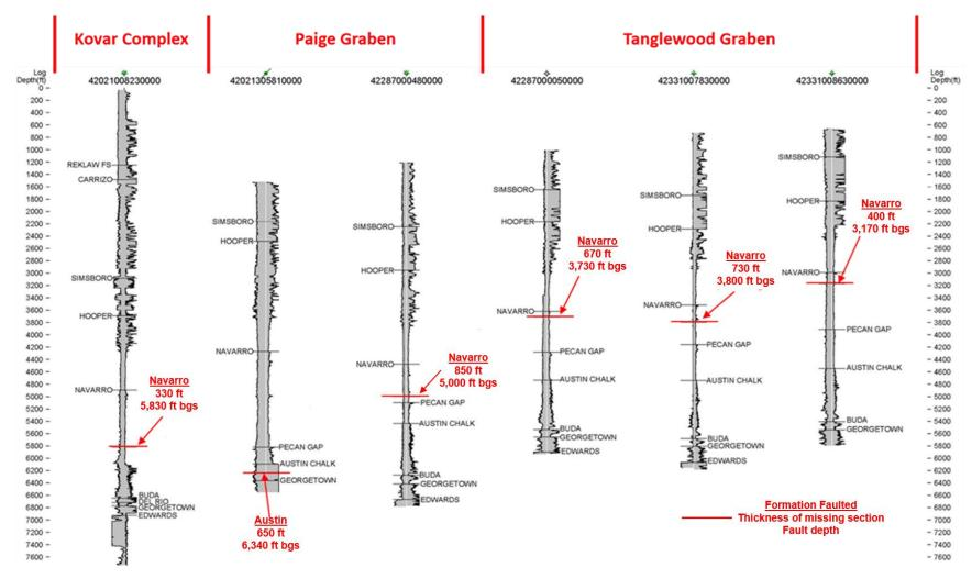
Figure 3.1.2d. Six logs containing fault cuts. Location of logs are shown in Figure 3.1.2g.
