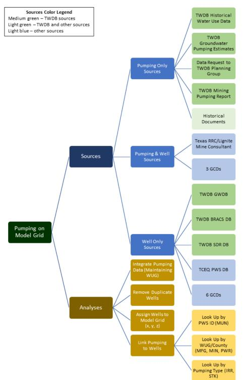
Figure 3.2a. Flow chart showing the data sources and analyses used to assign historical pumping to the model grid.
